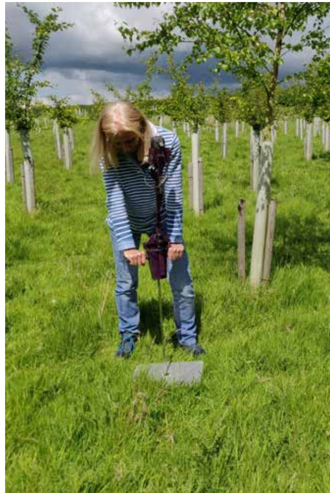
Measuring soil compaction using a penetrometer.
